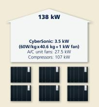
Through the use of CyberSonic, under the mentioned conditions the energy costs of the air conditioning can be lowered by 37,011€ (194,735€–157,724€). This constitutes a reduction in energy costs of 19 %, against an additional space requirement of 20 %.
