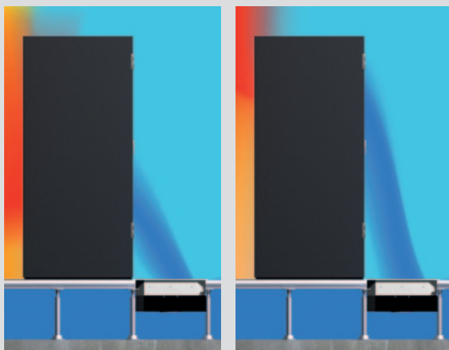
Manually adjustable air transfer grilles allow air flow to be directed to the most heat-stressed areas, depending on server rack equipment
